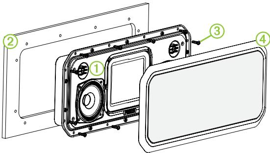
**14** If there is a concern that water may enter the mounting surface around the edges of the speaker, apply marine sealant around each of the screw holes and between the stereo and the mounting surface (optional).
