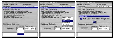
Num Pts menu with 5-point calibration selected (left). Half level selected on Fluid Level menu (center). Calibration completed window (right).
