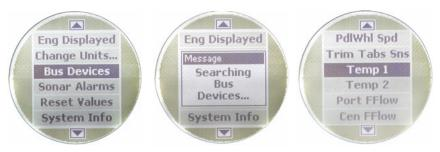
Bus Devices highlighted in the System Setup menu (left). Searching Bus Devices window (center) with Bus Devices list (right).
