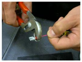
Attach appropriate connectors to wire leads.
