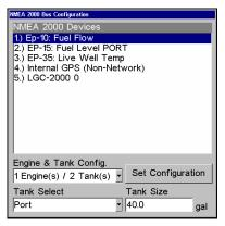
Bus Configuration menu with five items displayed on the NMEA 2000 Devices list. Engine-Tank Configuration and Tank Select menus are at the bottom of the screen.
