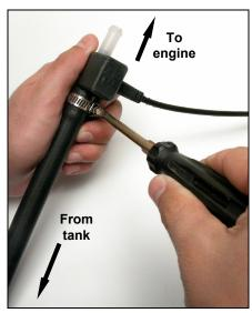
Push the fuel line onto the hose barb, then tighten the hose clamp. Orient the sensor vertically, with the flow arrow pointing up.
