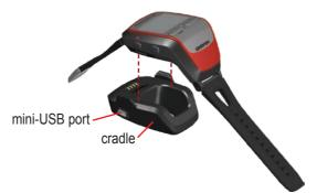
Plug the small end of the AC adapter into the mini-USB port on the cradle. Plug the other end into a standard wall outlet.
