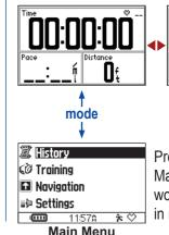
Press **mode** to view the Main Menu. Using the Main Menu, you can set up simple or advanced workouts, view your history data, save locations in memory, and customize the Forerunner.
