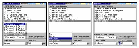
1 Engine/1Tank highlighted on Engine and Tank Configuration menu (left). Starboard highlighted on Tank Select menu (center). Tank Size set to 40 gallons (right).
