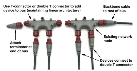
In this example, a new device is added to the NMEA 2000 bus by installing a T connector between a T connector and a terminator at the end of the backbone (network bus).
