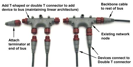
If you want to add a node at the end of the backbone (network bus) remove the terminator from the last connector, like the figure above. Install the new T connector, then attach the terminator to the side of the connector.
