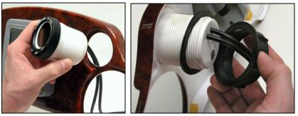
Insert gauge through the hole in the front side of the dash (left). Slide the rubber gasket over the cables, followed by the plastic collar (right).
